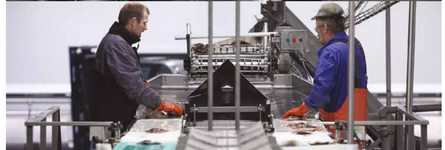
The fish are weighed and automatically sorted into 10 sizes on the grader and labelled with information on traceability and net weight before going to auction.
